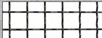
1-5/8" CENTER-TO-CENTER SQUARE 8 GAUGE WOVEN (1-1/2" SQUARE OPENING)
