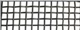
1/2" CENTER-TO-CENTER SQUARE 12 GAUGE WOVEN (3/8" SQUARE OPENING)
